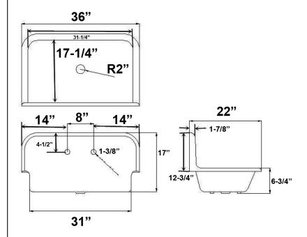
Dimensions of fixture are nominal and may vary within the range of tolerances established.
